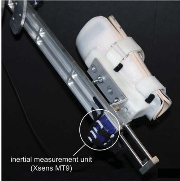
Fig. 3. Mounting of the inertial measurement unit on the exoskeleton's arm.
