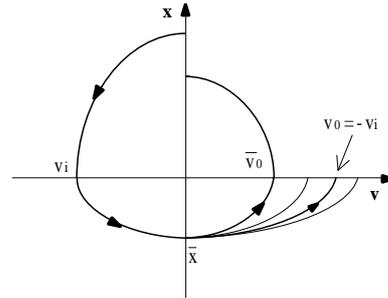
Fig. 2. Accessible set of output velocities by positive damping injection.
