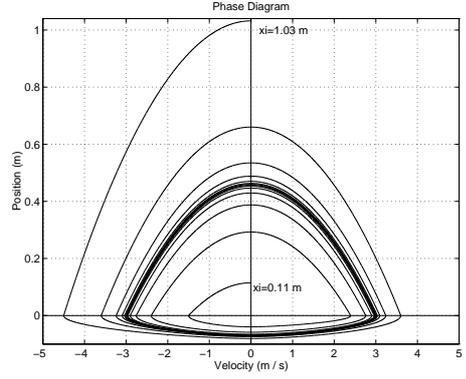
Fig. 5. Phase-plane motion with the asymptotic controller. The parameters for this simulations are:  $m = 1kg; n = 1; k = 1000N/m; x_d = 0.46m; \sigma = 0.4; \alpha = 0.3$
