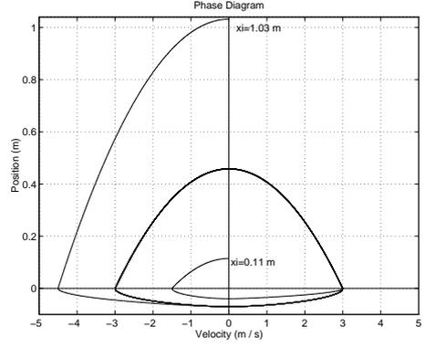
Fig. 4. Phase-plane for the dead-beat control. The parameters for this simulations are:  $m = 1kg; n = 1; k = 1000N/m; x_d = 0.46m; \alpha = 0.3$
