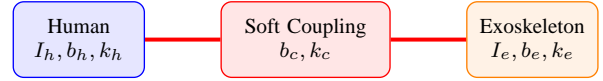
Fig. 3. Coupled human-exoskeleton system with soft coupling. Second-order linear models are used to represent the joint dynamics of the human (Eq. 1) and the exoskeleton (Eq. 2).
