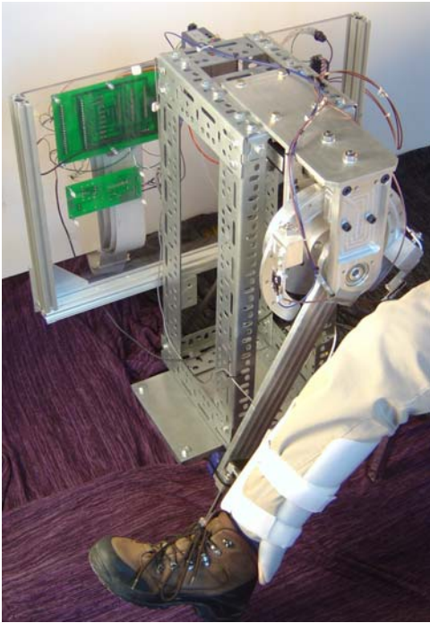
Fig. 3. 1-DOF exoskeleton for assisting knee-joint motion.
